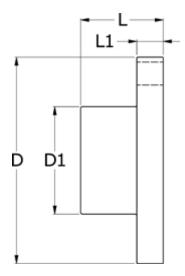
$\begin{array}{lll} D & = 252 \\ D1 & = 150 \\ L & = 100 \\ L1 & = 26 \\ Max bore & = 90 \\ Torque (N m) = 2750 \end{array}$
